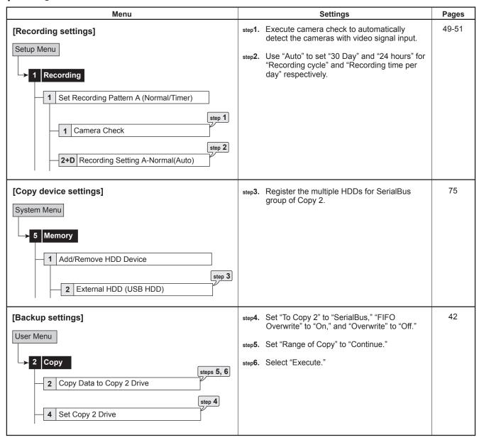
When setting the total capacity of the copy 2 device (registering the device) to larger than that of the main device, all the recorded data of the main device can be copied to the copy 2 device. In this operation example, the recorded data of more than one month in the main device can be stored to the copy 2 device. You can prevent the accidental erasure of the recorded data caused by the crash of the main device.
